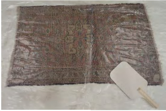
A test carpet being tamped
