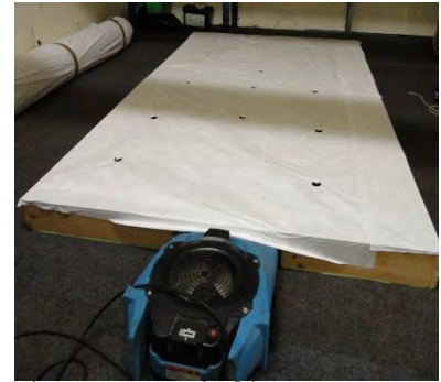
Tyvek covered drying platform
