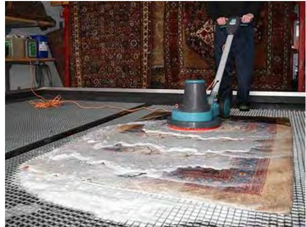
Rotary brush in use during a domestic rug wash.
