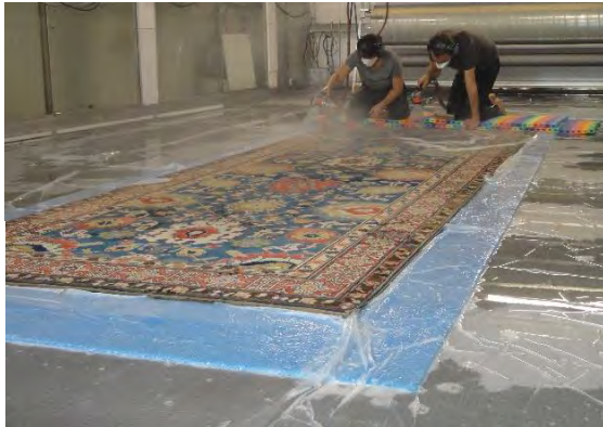
Washing flat with aerosol guns Image reproduced by kind permission of De Wit
