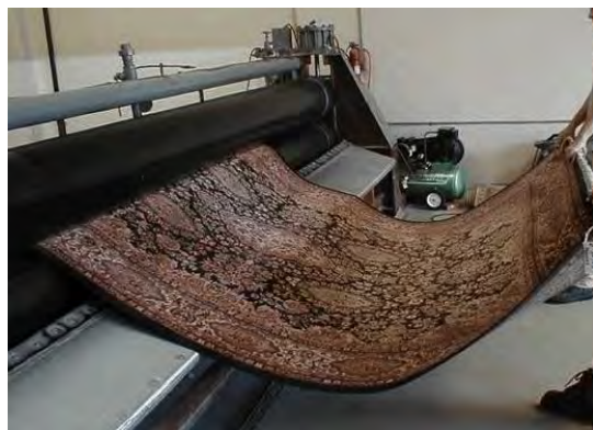
Press wringer or mangle in use
